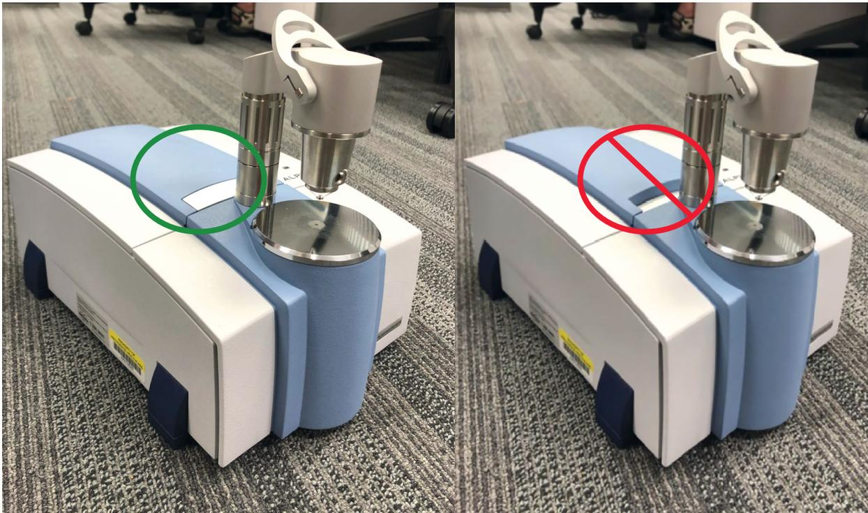
**Figure 3.** When the sampling module is properly secure, the rectangular button will be level with the spectrometer module (left).
